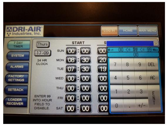
This keypad is used to enter all temperatures, times, and digital information. Press the desired numbers and then ENT to make the change.
