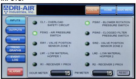
The inputs screen displays different sources of inputs, in this screen you can independently tell whether or not an input is on or off, as well as switching between auto and manual mode. This screen also displays an Hour Meter (Not resettable) and a Preventive Maintenance (PM) Meter (Which is resettable).
