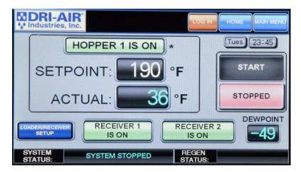
All common operator inputs are located on this main screen including starting and stopping the dryer, closed loop loader control and temperature changes. The asterisk (next to the setpoint) indicates the setback function is turned on. The setpoint temperature numbers change to red when the dryer is in setback.
