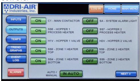
The outputs screen displays different sources of outputs, in this screen you can independently tell which output sources are on or off. You can also switch from Auto to Manual mode to test output operation.
