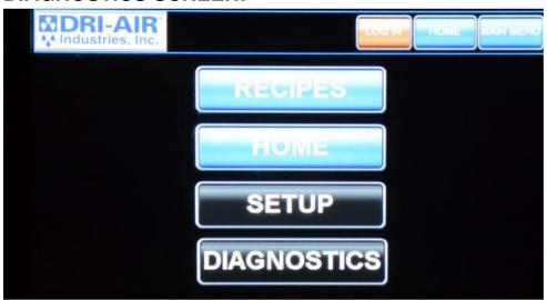
To enter the diagnostics screen, first tap the main menu button in the top right of the touch screen, and then select the "DIAGNOSTICS" button.
