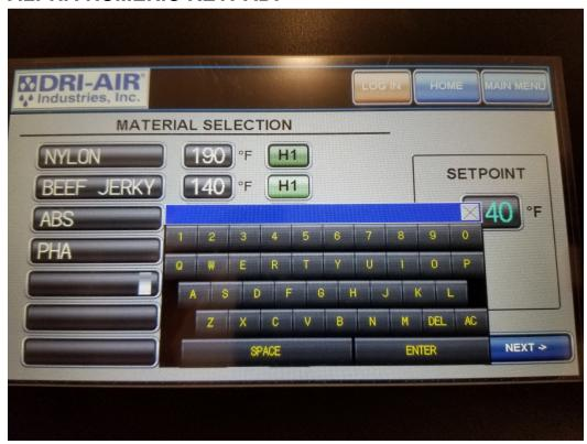
To enter a new recipe or other designation, press the center description area and the keypad as shown will appear. Type the new entry using the keypad and press enter.
